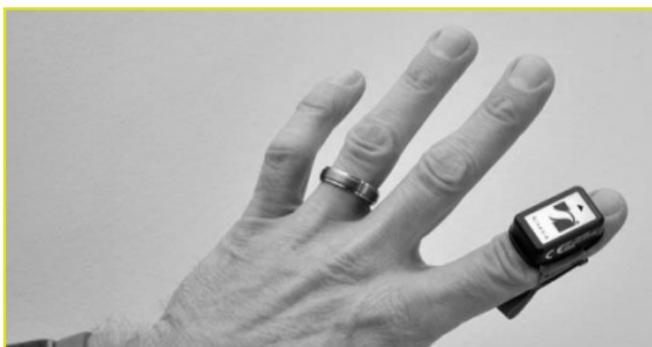
Kinesia Sensor to Measure Three-dimensional Movement
